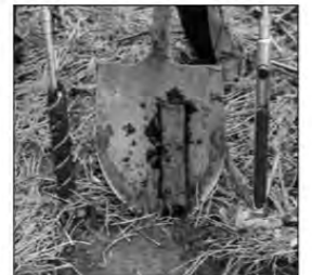
Figure 1. A soil probe, auger, or spade should be used in sampling soils. The spade sample (shown in the center of the picture) should be trimmed as shown with a knife.
